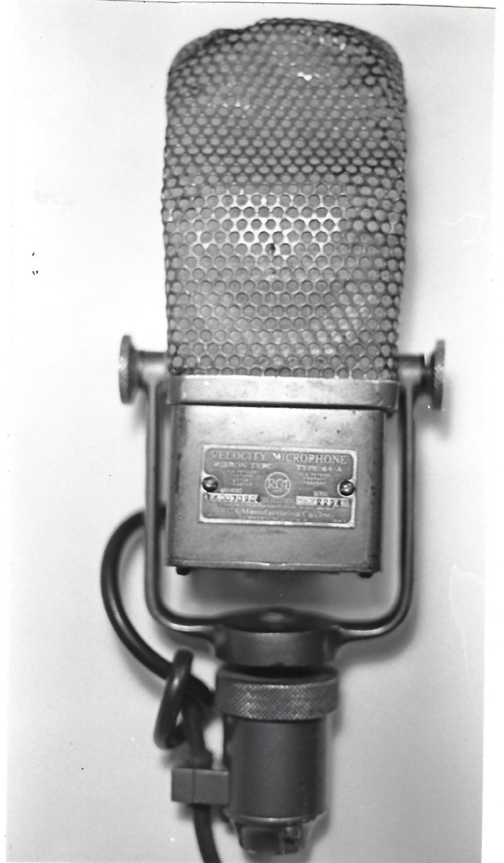
A close-up of the original ribbon type velocity microphone used (type 44-A) RCA
